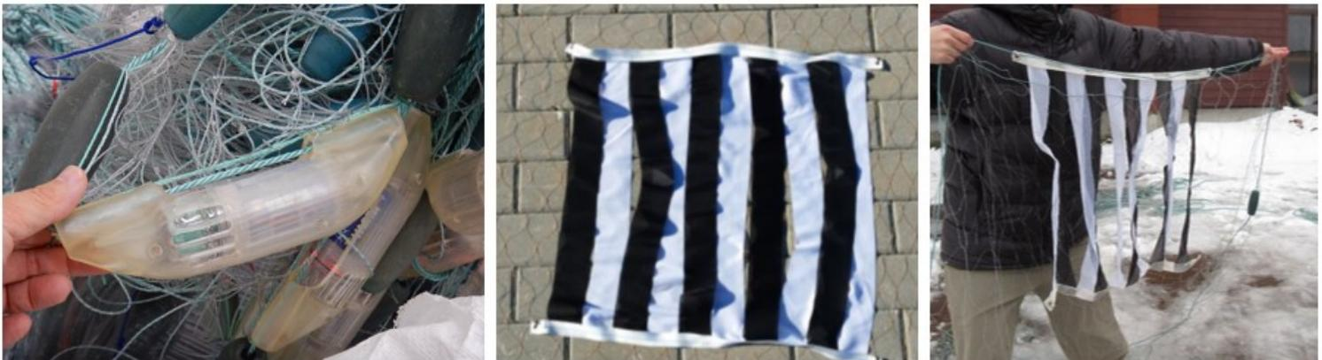
*Figure 2 - LED lights and light cases attached to an experimental gillnet (left), Striped fabric panel (center) and panels attached to an experimental net (right).*
