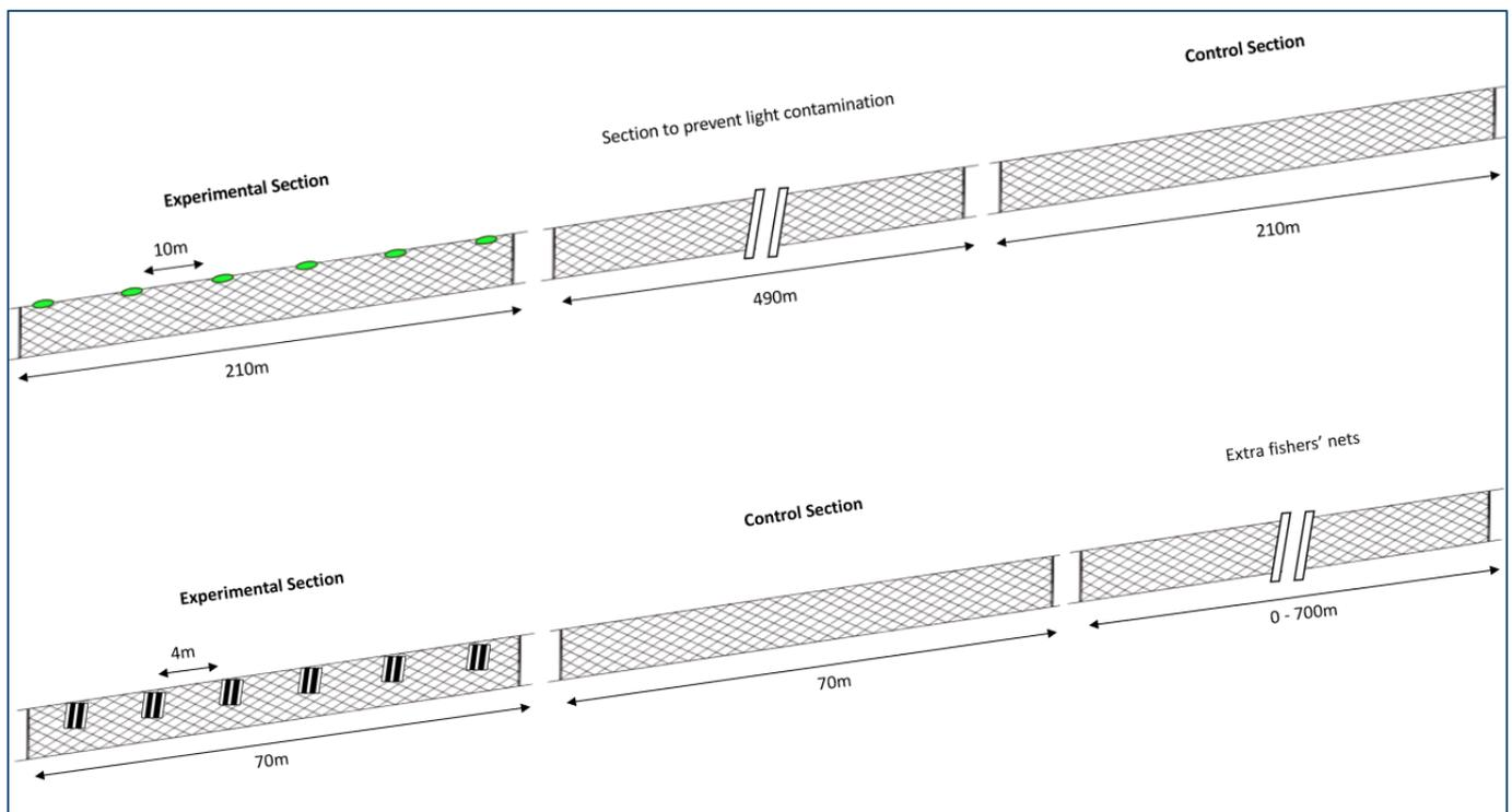
Figure 3 – Experimental set-up for gillnet trials; top diagram shows LED light set-up, the bottom diagram shows the high-contrast panel set-up
