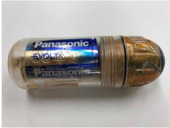
*Figure 8 – One of the non-functioning LED lights with rust visible inside the unit. When it was opened, some water ingress was apparent.*
